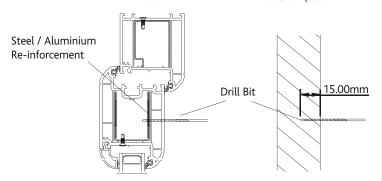
The two holes with washers underneath will require a 5mm drill bit. The three counter-sunk holes will require a 2mm drill bit.  $2 \times 5$ mm Drill Bit
