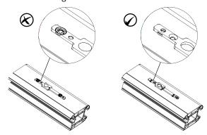
2 With the knocker bracket correctly located mark the fixing holes with a pen or pencil. 5 holes in total unless fitting a spyhole viewer.
