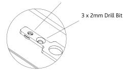
Place the bracket in the correct place with the two washers sitting over the 5mm drilled holes. Screw into place using 3.5mm PVCu screws into the three counter-sunk holes on the bracket.
