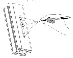
If available always use a drill punch to mark drilling positions using the pencil marks as a guide. The indent made by the point will ensure the drill does not slip.
