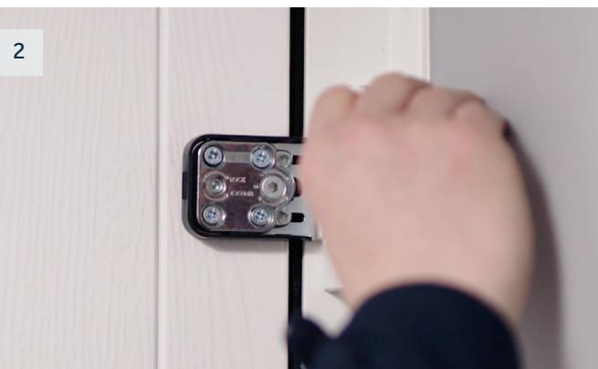
Once the cover is removed, use a 4mm Allen key to turn the unlock screw a  $\frac{1}{4}$  turn. Then, use the adjustment screw to adjust 5mm in either direction. When adjustment is complete, retighten the unlock screw, replace the hinge cover and fit the security screw back in. Repeat this process for all hinges.
